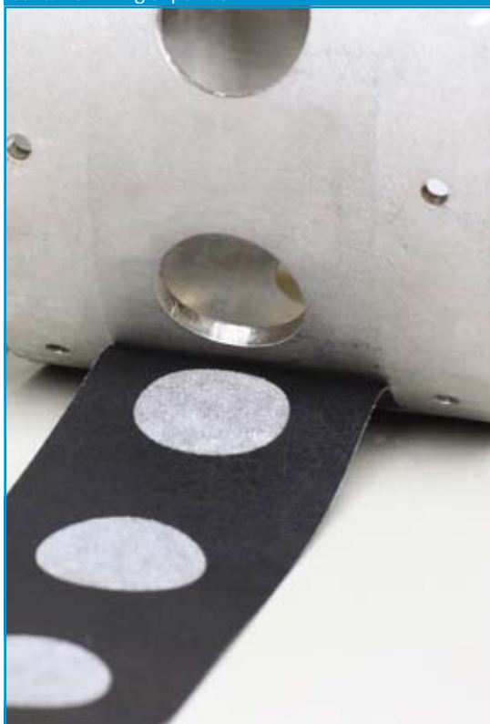
Figure 1: Each 2 cm diameter circle on this web contains 4.7 mg of powder.
